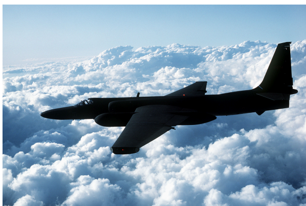
Lockheed U-2 high-altitude reconnaissance aircraft operated from the 1950s over Soviet territory and provided visual intelligence from an altitude of more than 20,000 metres in the era before satellites were widely available USAF (public domain)
