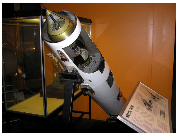
Bristol Thor ramjet engine of a Bloodhound Missile modified for display purposes at the (closed) Bristol Industrial Museum in 2004 Adrian Pingstone/Wikimedia, public domain
